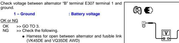
• Harness for open between alternator and battery (VQ35DE 2WD)
