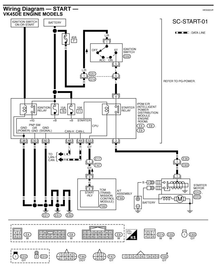
\*: THIS CONNECTOR IS NOT SHOWN IN "HARNESS LAYOUT", PG SECTION.
